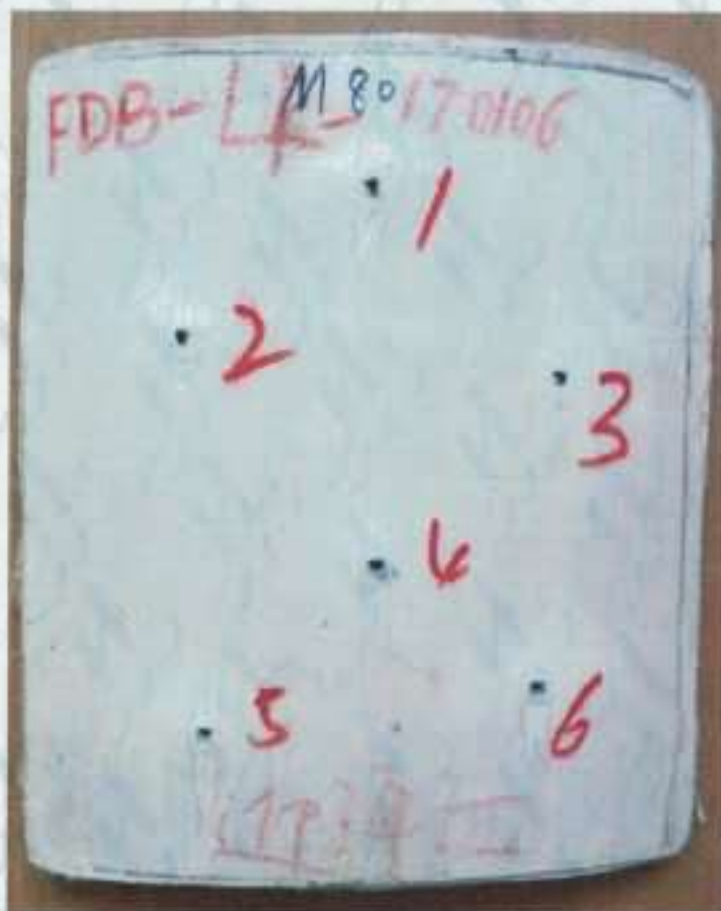
Fig. 1 Ballistic Insert FDB-LK-170106 (strike face)
