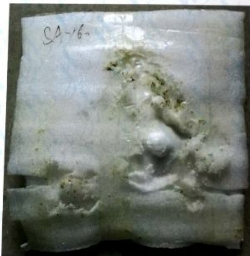
Fig. 2 Armor Panel SA-160 (wear face)
