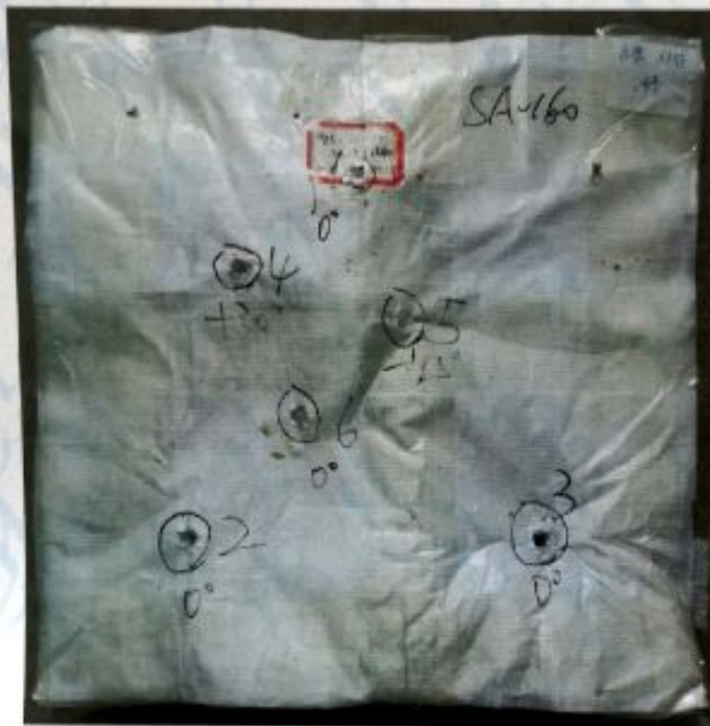
Fig. 1 Armor Panel SA-160 (strike face)
